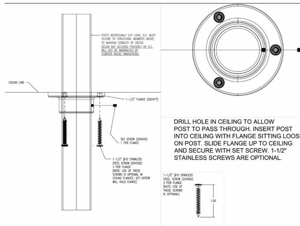
DRILL HOLE IN CEILING TO ALLOW POST TO PASS THROUGH. INSERT POST INTO CEILING WITH FLANGE SITTING LOOSE ON POST. SLIDE FLANGE UP TO CEILING AND SECURE WITH SET SCREW. 1-1/2" STAINLESS SCREWS ARE OPTIONAL.
