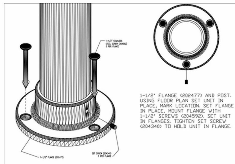
1-1/2" FLANGE (202477) AND POST. USING FLOOR PLAN SET UNIT IN PLACE, MARK LOCATION. SET FLANGE IN PLACE, MOUNT FLANGE WITH 1-1/2" SCREWS (204592). SET UNIT IN FLANGES. TIGHTEN SET SCREW (204340) TO HOLD UNIT IN FLANGE.
